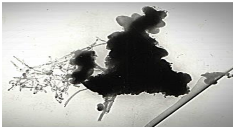
Figure 2 – TEM images of the 49.95% Ni + 49.95% Al + 0.1% Pt catalyst.
